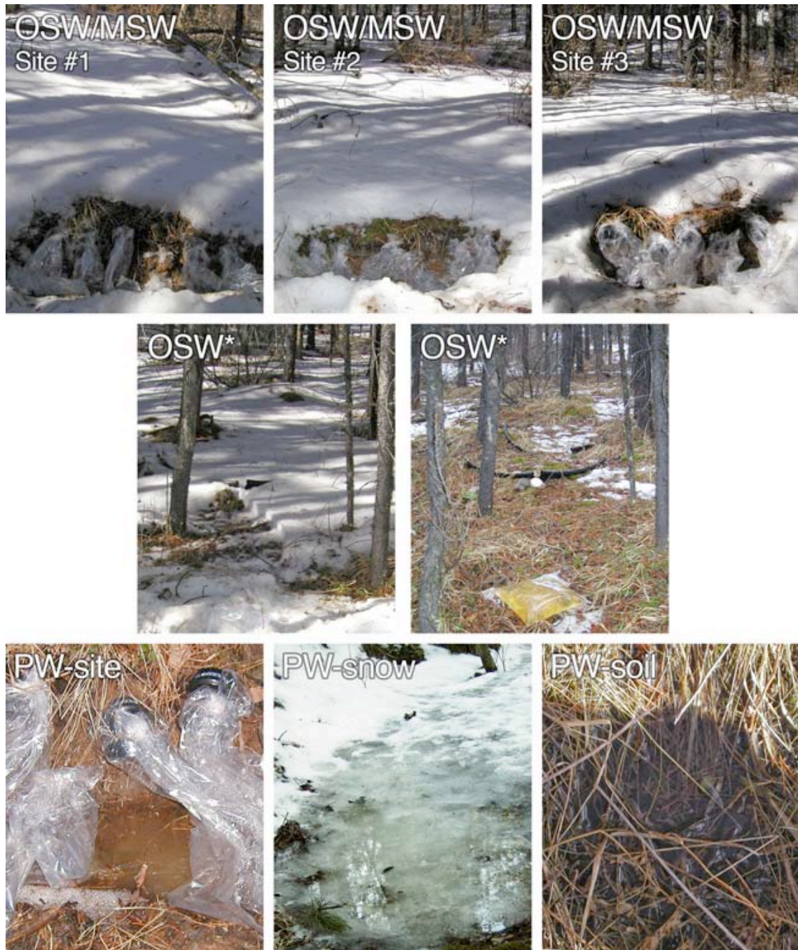
Figure 7.4. Photographs of sampling sites. Top row: the individual collection sites at the observation site for organic soil water (OSW) and mineral soil water (MSW). The numbers refer to position on the slope (see Figure 7.1). Centre row: overland flow installation close to site #3 where water was present during the rain-on-snow event (OSW*). Bottom row: collection sites for ponded water; in the depression in front of the lysimeter transects (PW-site) as well as on top of snow (PW-snow) and soil (PW-soil) in the vicinity of the observation site.
